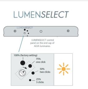
The LumenSelect rotary switch should be turned gently clockwise with a small flathead screwdriver with a 1/8" or 3mm wide tip, one click at a time from factory setting to get desired output level.
